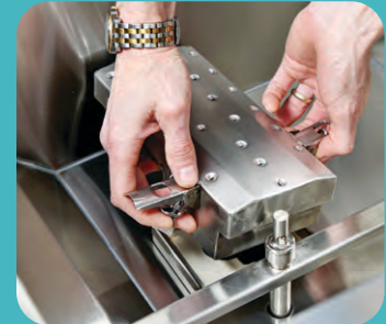
Stationary spray box simply unlatches for easy visual inspection and cleaning.
